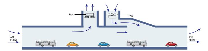
■ 6. Point Extraction Type Longitudinal Ventilation (PEV)
